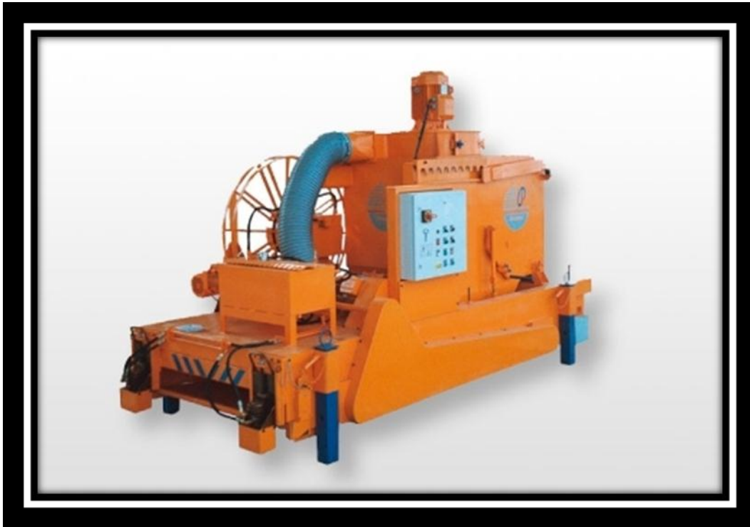
WIRE PULLING MACHINE: PRESTRESS CABLE LAYING
